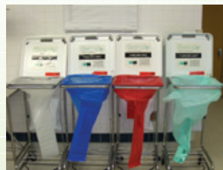
ORs at Inova Fairfax are now equipped with containers for solid waste (clear), linen (blue), regulated medical waste (red) and recycling (green).
