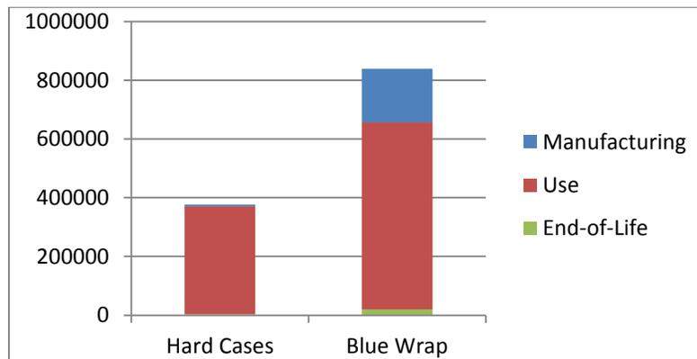
Figure 2: 10-year totals and proportions of manufacturing, use, and end-of-life phases.
